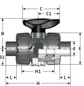
With secured union nuts and threaded sockets with threaded connection.
