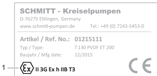
Fig. 2 ATEX type plate (example)
