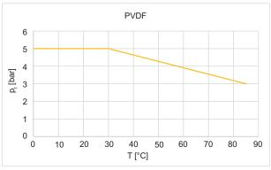
Fig. 10 Total pressure, pump head material PVDF
