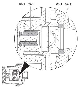
Fig. 6 Components of the plain bearings
