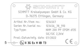
Fig. 2 ATEX type plate (example)
