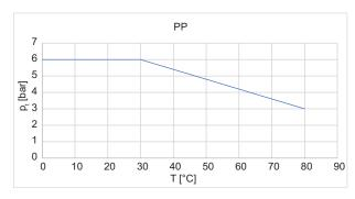
Fig. 9 Total pressure, pump head material PP
