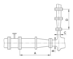
Fig. 5 Straight pipe lengths in front and after the pumps (recommended)
